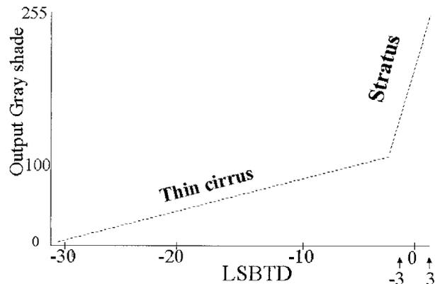
FIG. 1. Graph of enhancement used for TLE. LSBTDs of  $-30$  to  $-3$  K are mapped to output gray shades of 0–100. LSBTDs of  $-3$  to  $+3$  K are mapped to 101–255.
