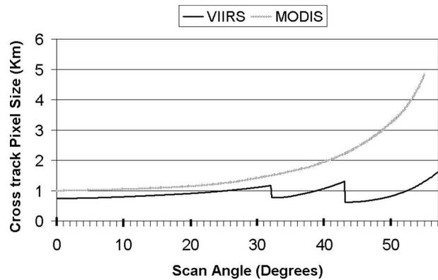
FIG. 4. Comparison of 1-km (nadir) resolution used for 29 of 36 MODIS channels with 0.76-km (nadir) resolution for VIIRS at moderate resolution. Of the 22 VIIRS channels, 17 use the resolution shown here. Five use a higher resolution of 0.38 km (nadir).
