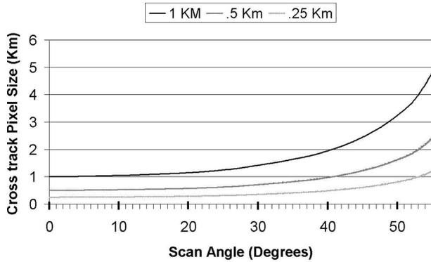
FIG. 1. MODIS cross-track variation in pixel size as a function of scan angle away from nadir. Half- and quarter-kilometer data are used in construction of true-color images.
