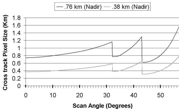
FIG. 2. VIIRS cross-track variation in pixel size as a function of scan angle away from nadir. Both resolutions will be used in the construction of true color.
