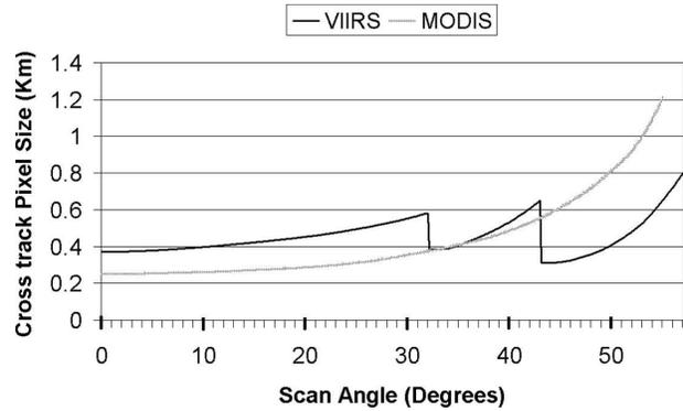
FIG. 3. Comparison of cross-track pixel size for high-resolution red input channels required for true color: VIIRS 0.38-km (nadir) resolution vs MODIS 0.25-km (nadir) resolution.
