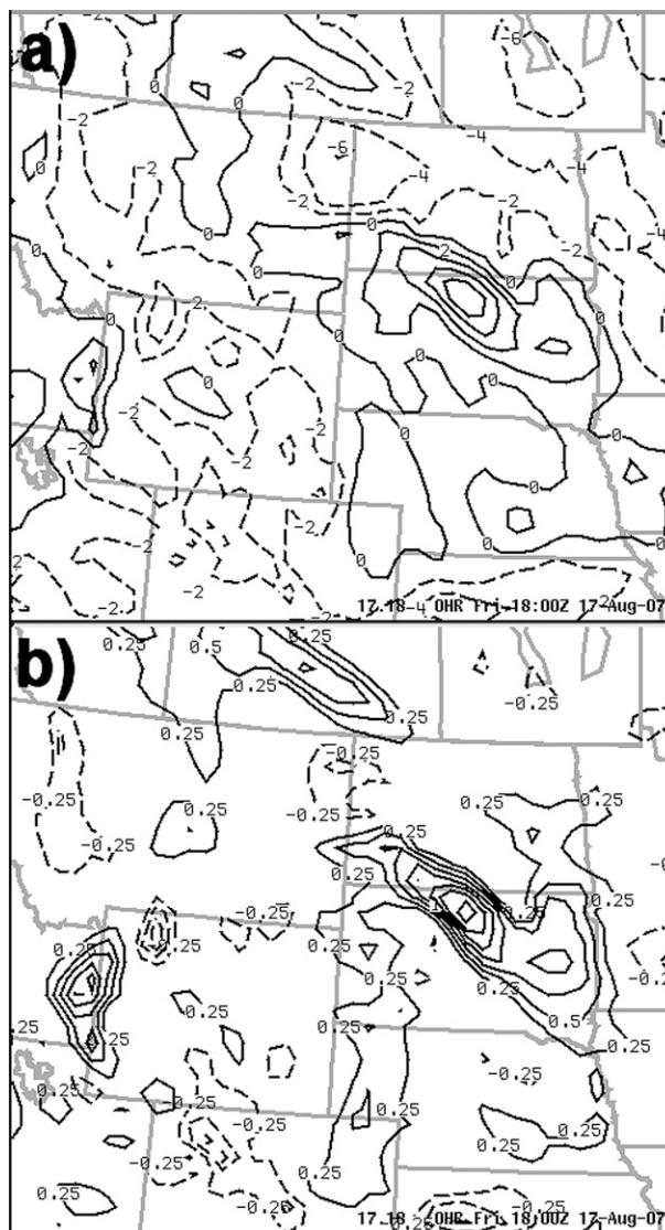
FIG. 1. Plot of the (a) MCS index and (b) 700-hPa TAdv valid at 1800 UTC 17 Aug 2007 from the 40-km RUC. Contour intervals are 2 for the MCS index (dashed negative) and  $0.25^\circ \text{C h}^{-1}$  for TAdv (dashed indicates negative; zero contour is omitted).
