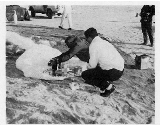
FIG. 3. Balloon-skin temperature and balloon vertical acceleration instrumentation on the valving plate.
