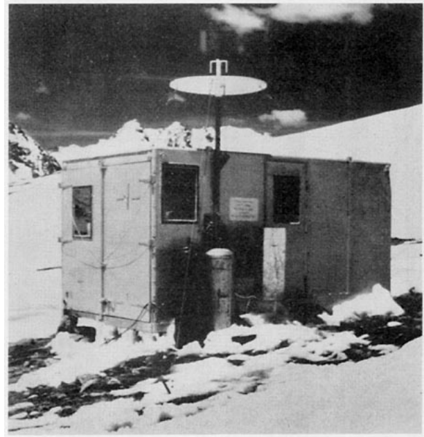
FIG. 1. Data collection platform on Niwot Ridge, Colorado, 3536 m.
