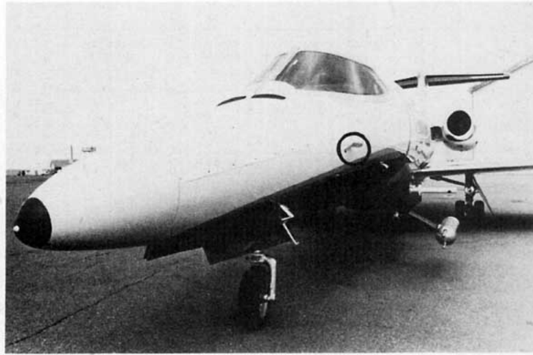
FIG. 1. Photograph of Colorado International Corporation (CIC) Learjet showing angle of attack vane (circled) and door pod with research instrumentation (behind).
