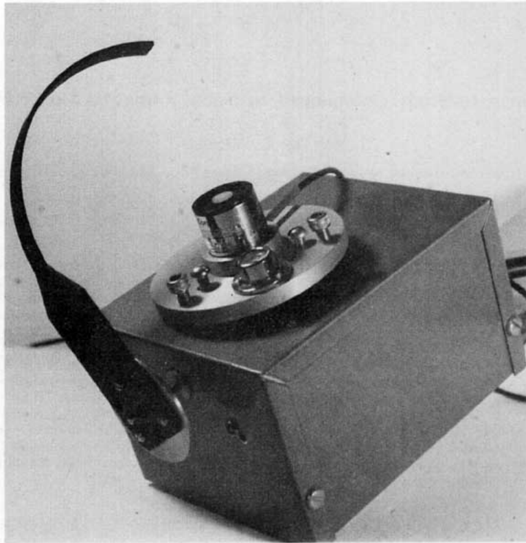
FIG. 1. The dial assembly with a cosine-corrected silicon sensor in place beneath the occulting strip. The actual sensing area to be shaded is the white disk at the center of the radiometer head. In use, the device is leveled and mounted so that the occulting arm can pass under the box.
