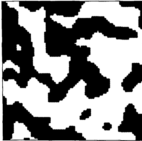
FIG. 2. The simulated cloud pattern for the model that gives a well-defined scale of correlation. An array of random numbers was smoothed with a Gaussian function (to make a correlated array) and then truncated to simulate clear-sky and cloud-covered pixels. Since there is no finescale variation, the edges are sharp, and therefore the pattern does not look intuitively "cloudlike."
