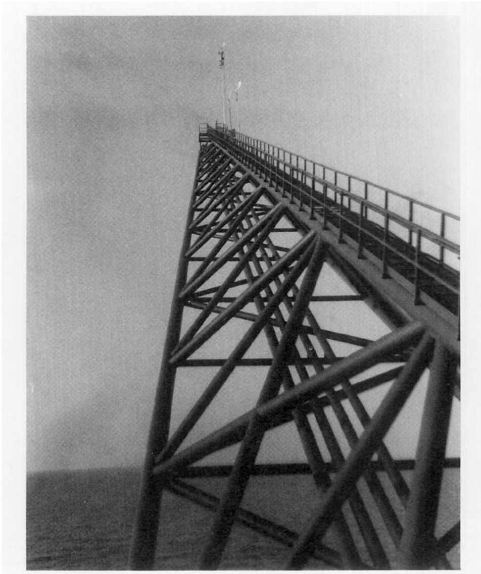
FIG. 3. A close-up view of the C-MAN anemometer system on the boom of station GBCL1. Note that the dual-anemometer system was installed on the station so that one of them could act as a backup.
