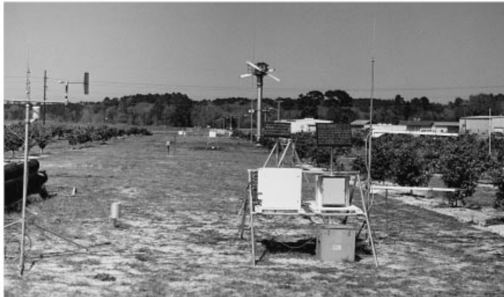
FIG. 2. Top panel provides a schematic illustration of a SREBS system; the temperature measuring arms are placed at 1.5 and 2.5 m above the surface. Bottom panel provides a photograph of the two SREBS systems deployed in the IFAS experimental orchard. The station closest to the camera is the south station, while the north station is barely visible at the other end of the grove.
