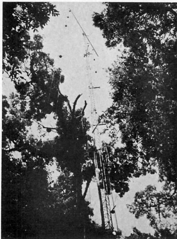
FIG. 4. Instrumented 200-ft tower in the jungle.
