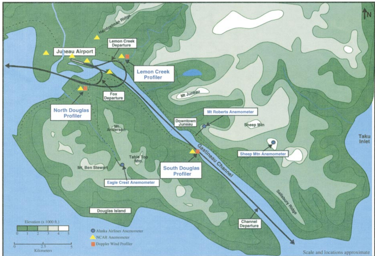
FIG. 1. Topographic map of the Juneau, AK, area. Wind profilers are located at Lemon Creek, South Douglas Island, and North Douglas Island. The three aircraft departure patterns are known as the Fox, Lemon Creek, and Channel departures.
