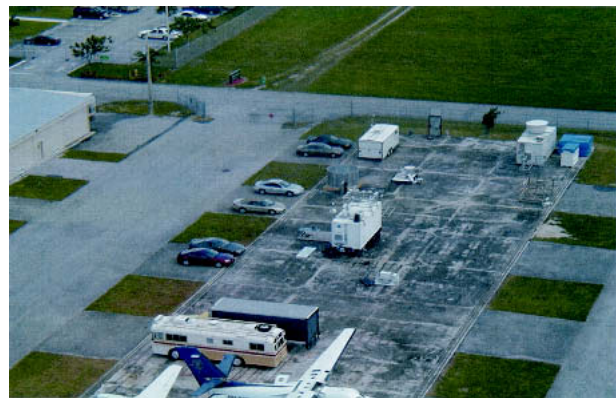
FIG. 1. Aerial photograph of the eastern CRYSTAL FACE field site at the Kendall-Tamiami Executive Airport near Miami, where (clockwise from the top right of the tarmac) the roof-mounted NOAA K-band Doppler radar, the NASA Surface Measurements for Atmospheric Radiative Transfer (SMART) van that held the MPL and several radiometers, the circular rain guard enclosing the NOAA S-band radar dish, and the free-standing University of Miami W-band Doppler radar attached to its supporting van are shown.
