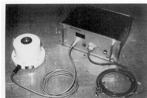
FIG. 1. Photograph of a set of MCP: on the left the sensor, on the right the controller.
