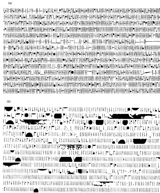
FIG. 5. (a) 2D-P images for the period 1058:27–1058:54 UTC during a melting layer study conducted on 22 May 1986 near Boston. Vertical separator bars represent a scale of 6.4 mm. (b) 2D-C images obtained during the same time interval as the 2D-P images in (a). Image separators here represent a scale of 0.8 mm.
