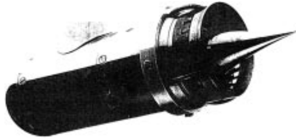
FIG. 2. M-meter prototype in operating configuration. It is 6 cm in diameter, 20 cm long, and has a mass of 1.4 kg.
