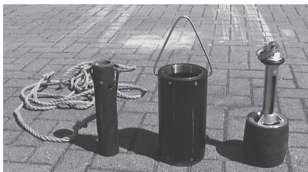
FIG. 1. Examples of SST buckets in current use by the VOS of (left) the United Kingdom, (middle) the Netherlands, and (right) Germany.
