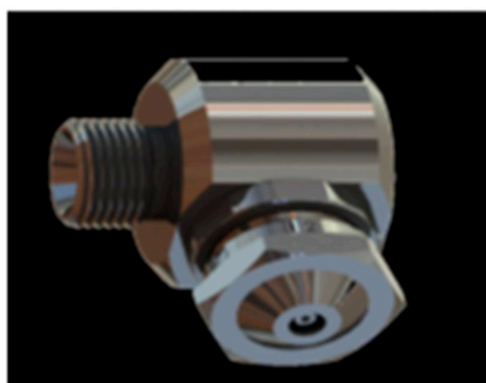
FIG. 7. The Schlick model 940 form 6 two-fluid nozzle used for spraying crudely fluidized Albalfil T10: (left) photograph and (right) detail drawing. The fluidized material enters via the liquid inlet, passes through the center of the liquid insert, and exits through the smaller of the apertures seen in the photograph. Compressed air enters via the air inlet, swirls around the outside of the liquid insert, and exits through the larger of the apertures.
