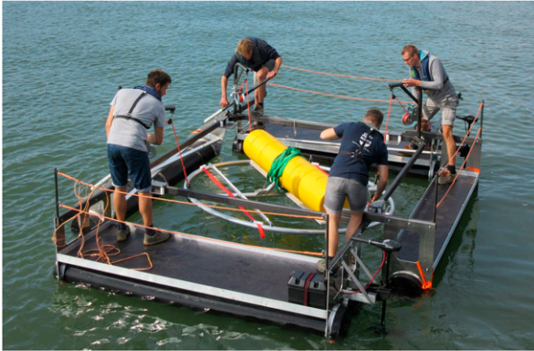
FIG. 8. Test of the small-rings-to-cable-network assembly raft in the NIOZ harbor.
