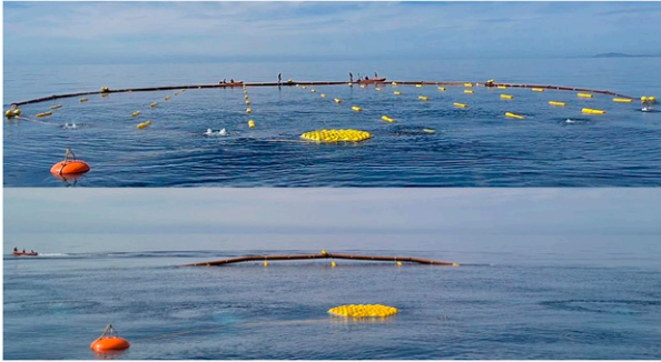
FIG. 10. Two video stills from the final minute of valve opening before sinking of the 3D-T mooring array.
