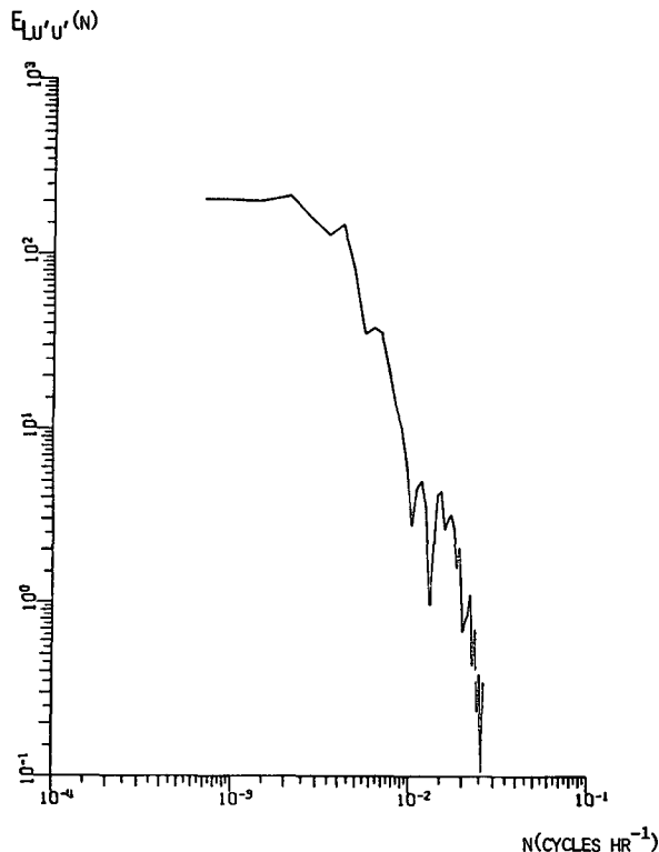
FIG. 3. Normalized energy spectrum of the zonal velocity of individual particles.
