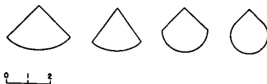
FIG. 2. Conical models: left to right—90° cone-spherical sector, 70° cone-spherical sector, 90° cone-hemisphere and 90° teardrop.
