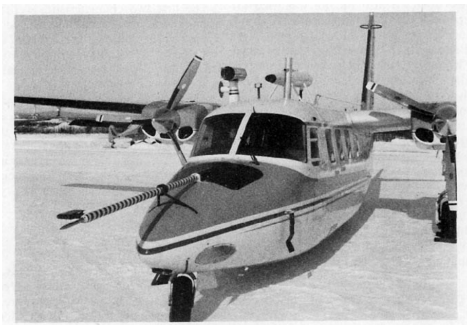
FIG. 3. The instrumented aircraft used for sampling clear-sky ice crystals.
