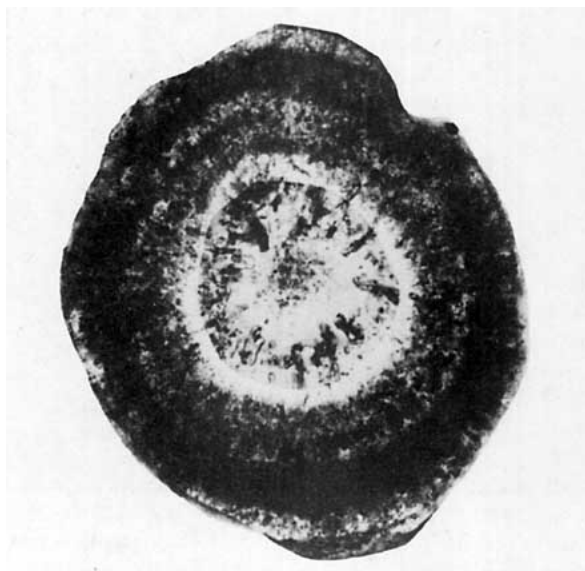
FIG. 15. Thick section of a hailstone whose graupel embryo is substantially transformed by soaking and/or melting. The D and O^{18} measurements show that evaporation takes place out to the layers marked by the change in illumination, introduced artificially. The outer layers show condensation.
