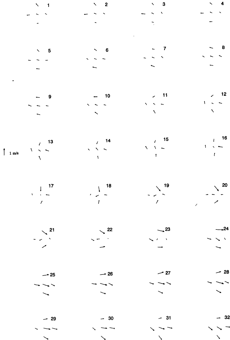
FIG. 5. Horizontal wind field for the 32 bins after the ensemble-averaging procedure. The propagation direction is from left to right. The arrows are based at vertices and center of the experimental square.
