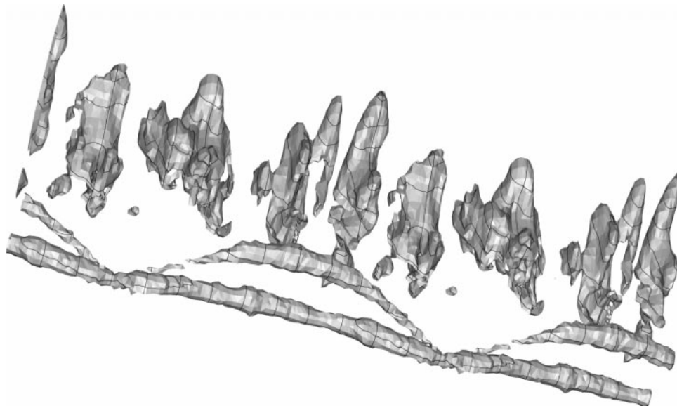
FIG. 13. Three-dimensional isosurface of ice crystal surface area density = 0.005 \text{ m}^{-1} for a simulated B747 contrail with RH_i = 110\% and shear = 0.01 \text{ s}^{-1} (simulation A10d) at an age of 90 s. The downstream domain length shown is 600 m.
