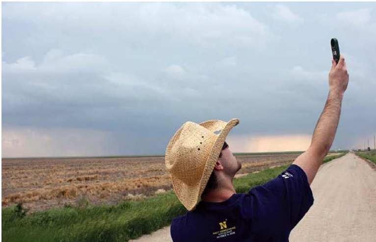
Fig. 2. Taking surface temperature and dewpoint temperature observations near Goodland, Kansas, on 23 May 2010 with a Kestrel 3500 ten minutes before tornado touchdown.
