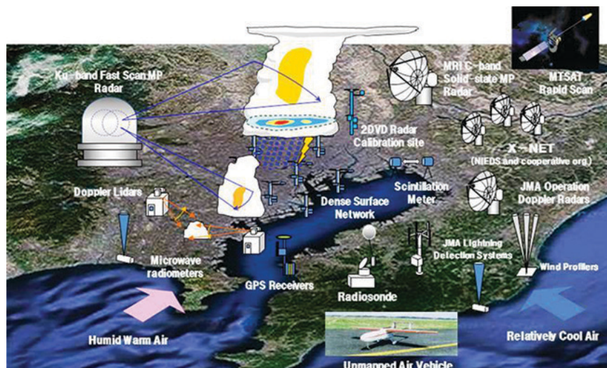
FIG. 1. Observation instruments in the TOMACS field campaign (after Nakatani et al. 2013).
