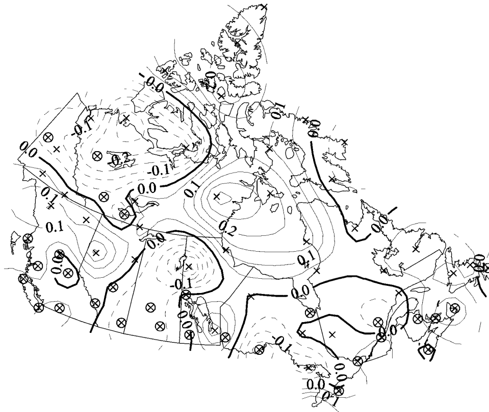
FIG. 1. Trend (1940–95) in the fraction of annual precipitation falling in the largest 10% of daily events (from Mekis and Hogg 1999). Stations that commenced data collection after 1940 and prior to 1910 are marked with black crosses and circled crosses, respectively. Unit is \% \text{ year}^{-1} of the annual total.
