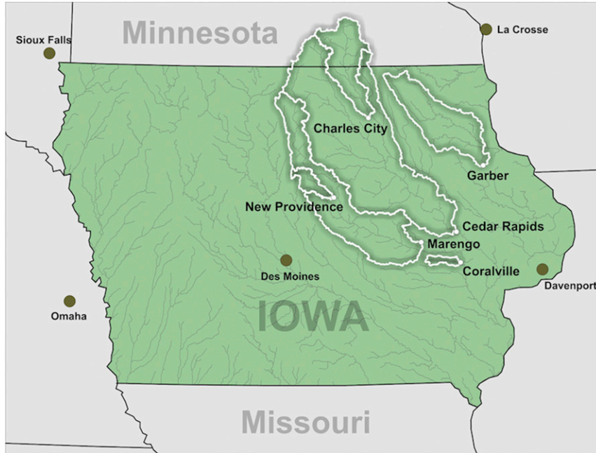
FIG. 4. Location of the six catchments considered in this study. The white circles at the outlets show the location of the USGS stream gauges. Brown circles show the location of the weather radars.
