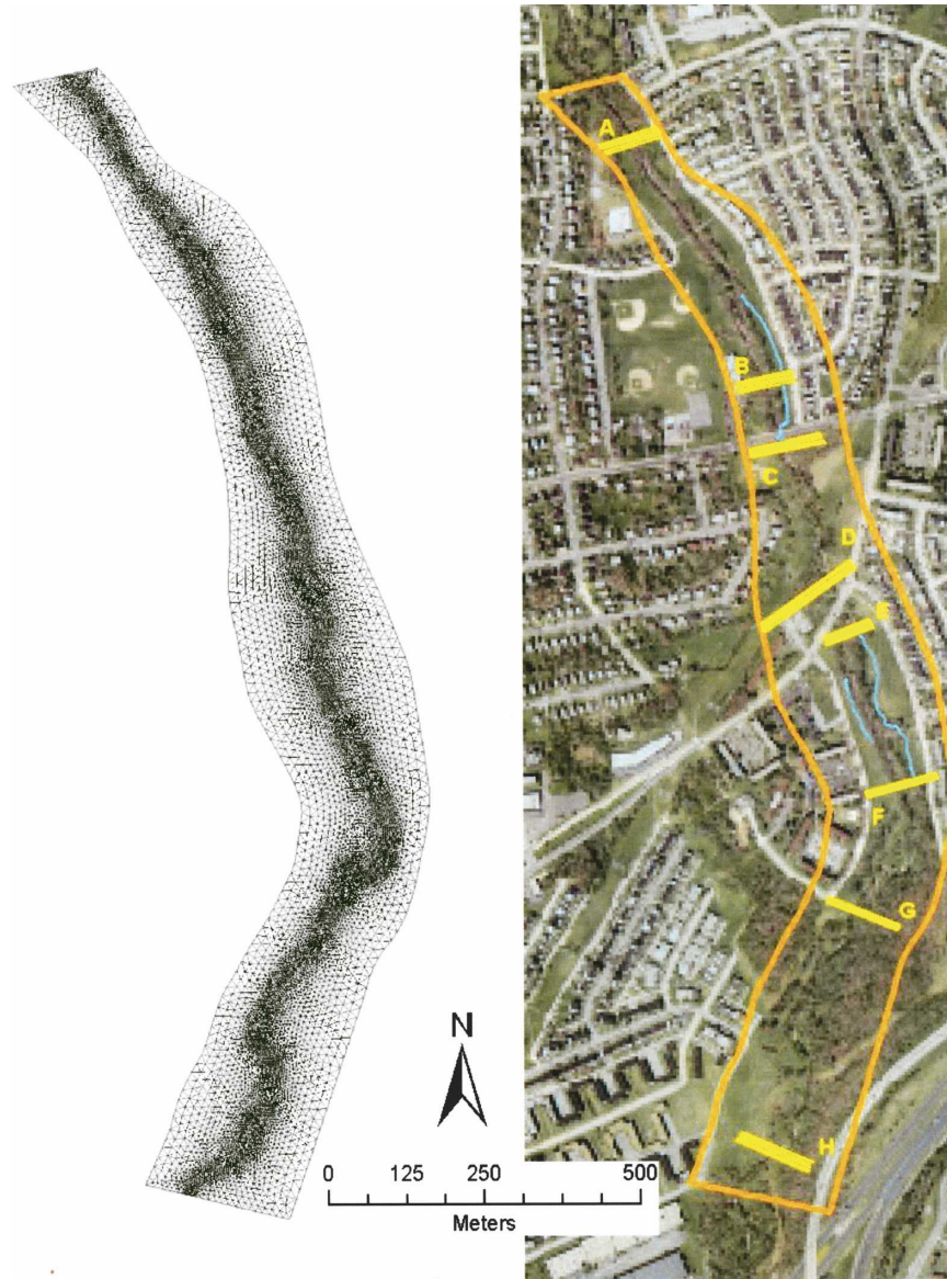
FIG. 11. (right) Aerial photograph of the Moores Run channel reach used for hydraulic model analyses. (left) The finite element mesh used for model analyses. Cross sections for which discharge times series are computed (see Fig. 14) are marked by the letters A–H. The Radecke Ave. Bridge is located between cross sections B and C. The Sinclair Ave. Bridge is located between cross sections D and E. Lines along which dense high-water mark observations were made are shown above Radecke Ave. Bridge and downstream of Sinclair Ave. Bridge.
