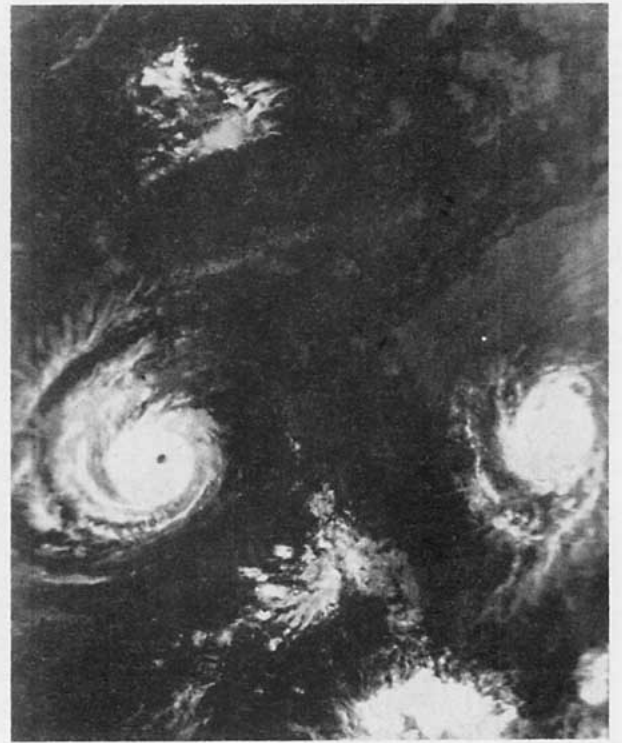
FIG. 3. Infrared data corresponding to Fig. 2. White represents effective radiating temperatures of 190K or colder, and the darker shades represent progressively warmer temperatures.
