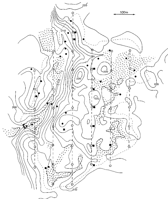
FIG. 1. Map of the Usadievskiy catchment at Valdai. Water-table measurement sites are indicated by filled circles. Soil moisture measurement sites are indicated by filled squares. Open circles with dashed lines indicate the snow measurement sites and routes, respectively. Runoff is measured at the stream outflow point of the catchment located in the lower left-hand corner of the map and indicated by a bold bracket. The short dash line denotes the catchment boundary. Hatched areas denote regions of swampy conditions. Elevation contours are in increments of 2 m.
