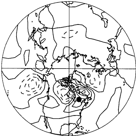
FIG. 4. Analysis increments from single observation experiment, where +3 \text{ J kg}^{-1} \text{ K}^{-1} observation increment in \pi was induced at location designated by dot. Contours every 0.01 \text{ J kg}^{-1} \text{ K}^{-1} . Negative increments dashed. (a) 400-member ensemble, (b) 25-member ensemble.
