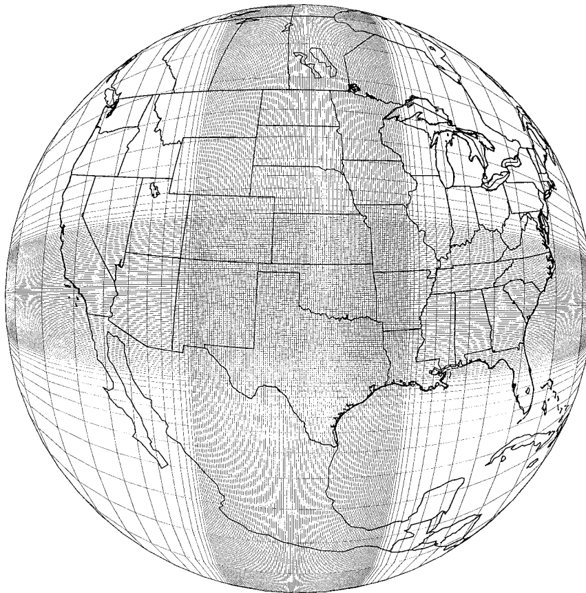
FIG. 6. The 353 \times 415 -point grid used for the VORTEX case with a 240 \times 323 -point uniform resolution ( 0.04^\circ ) window. For clarity every third point in each direction is plotted.
