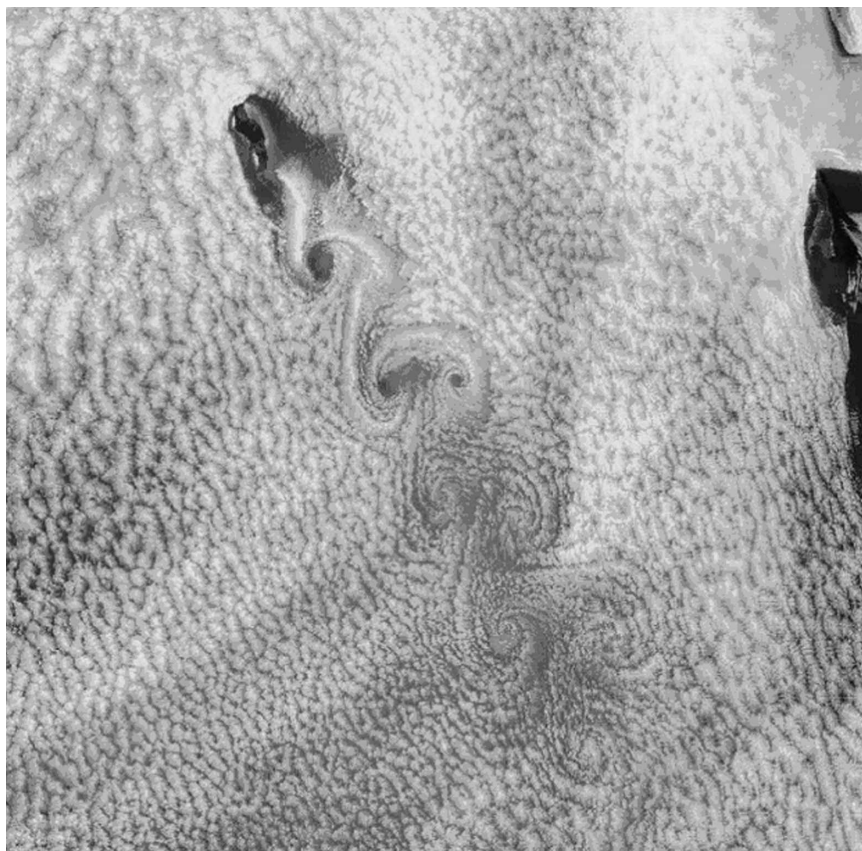
FIG. 1. A von Kármán vortex street in the stratocumulus off the island of Guadalupe at 1845 UTC 13 Jun 2004. The image was taken by the Terra MODIS satellite. Image courtesy of MODIS Rapid Response Project at NASA GSFC.
