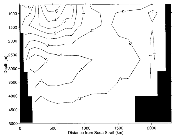
FIG. 14. Annual mean total velocity below 700 m across IX1 section from the model. Shaded areas denote flow from the Indian to Pacific Oceans. C.I. = 1 \text{ mm s}^{-1} .
