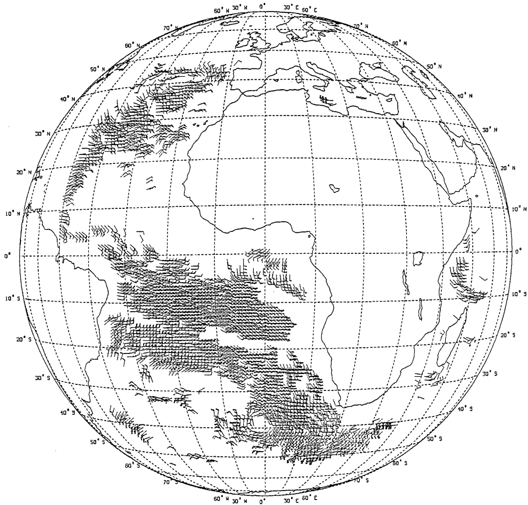
FIG. 4. Wind vectors derived from tracking clouds in high-resolution VIS images on 28 September 1995, 1130 UTC (see Fig. 1). A total of 2927 low-level vectors has been obtained.
