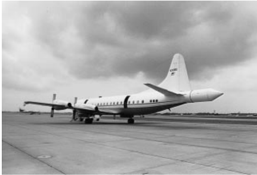
FIG. 11. The NCAR Electra aircraft outfitted with ELDORA at Oklahoma City during VORTEX-95; the antenna is mounted in the tail section (copyright H. Bluestein).
