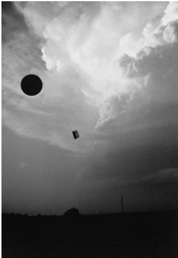
FIG. 2. Radiosonde just launched from an OU intercept vehicle upstream from a developing severe convective storm in western Oklahoma on 6 May 1986 (copyright H. Bluestein).
