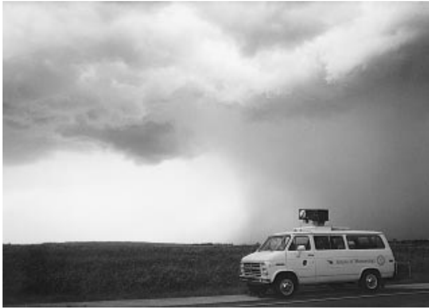
FIG. 8. The University of Massachusetts mobile 3-mm wavelength Doppler radar system mounted in an OU van, probing a convective storm on 7 Jun 1993 in central Kansas (copyright H. Bluestein).
