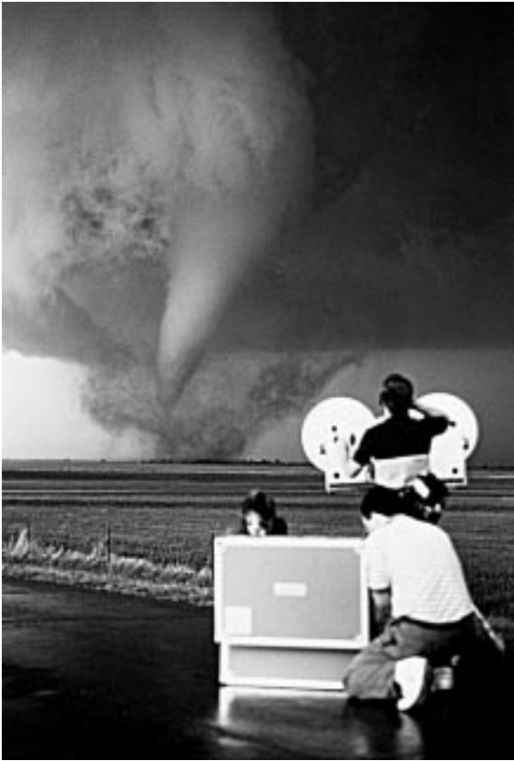
FIG. 6. OU students probing a tornado north of Enid, OK, on 12 Apr 1991, with the LANL portable Doppler radar (copyright H. Bluestein).
