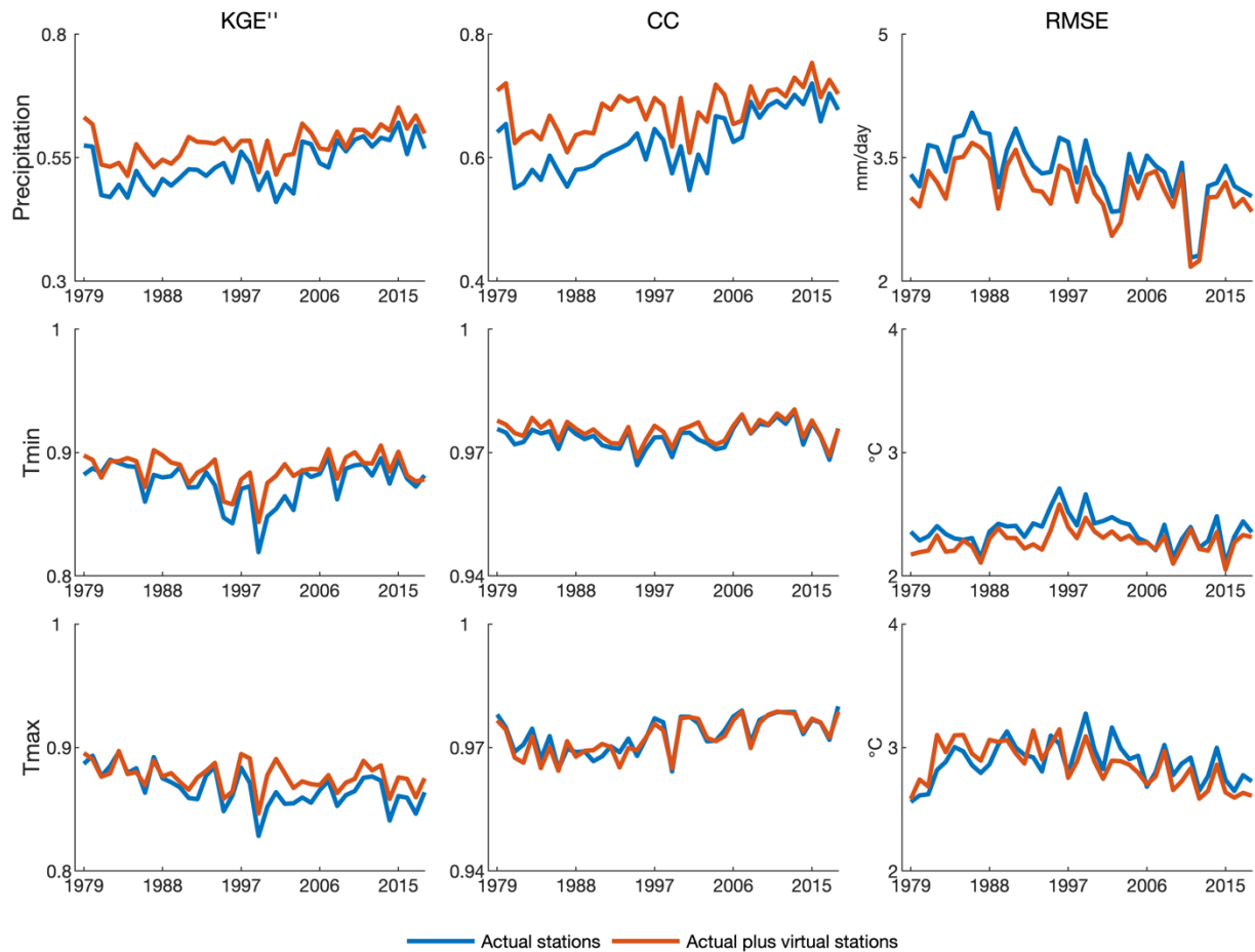
Figure S6. KGE'' , CC and RMSE for interpolated precipitation, Tmin and Tmax estimates from 1979 to 2018. Median values of all stations are used for every year. The interpolation method is IDW.
